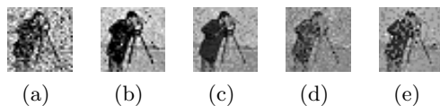
Fig. 3. Extracted watermarks under different signal processing attacks. (a) Gaussian noise, (b) histogram equalization, (c) JPEG compression, (d) median filtering, and (e) cropping.
