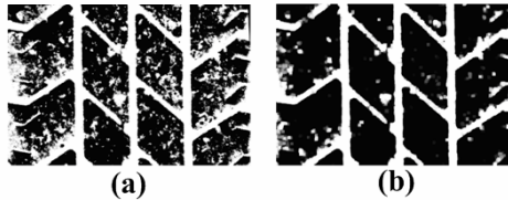
Fig. 2. (a) Original tire image, (b) Result after image preprocessing procedures
