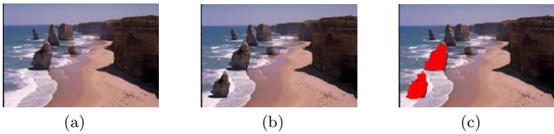
Fig. 7. Detection of a scaled-copied rock: (a) original, (b) tampered with the rock shrunk by 0.8 and pasted, and (c) detection result
