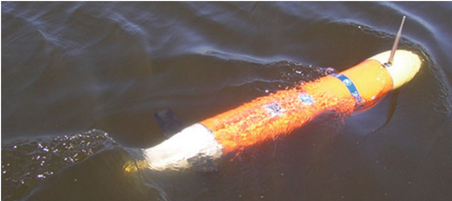
Fig. 3.13 Light Autonomous Underwater Vehicle (LAUV).
