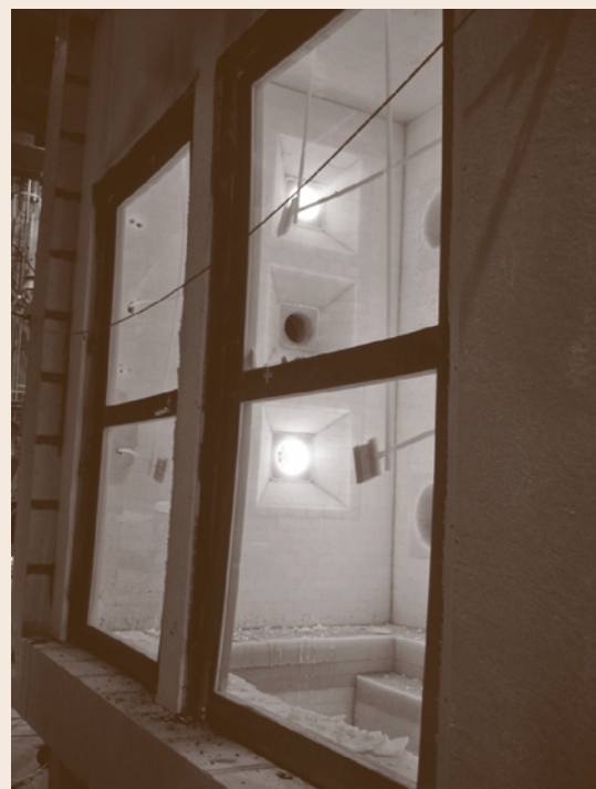
Fig. 15.35 Fire-resistance testing of a glazed partition (courtesy of SP)
