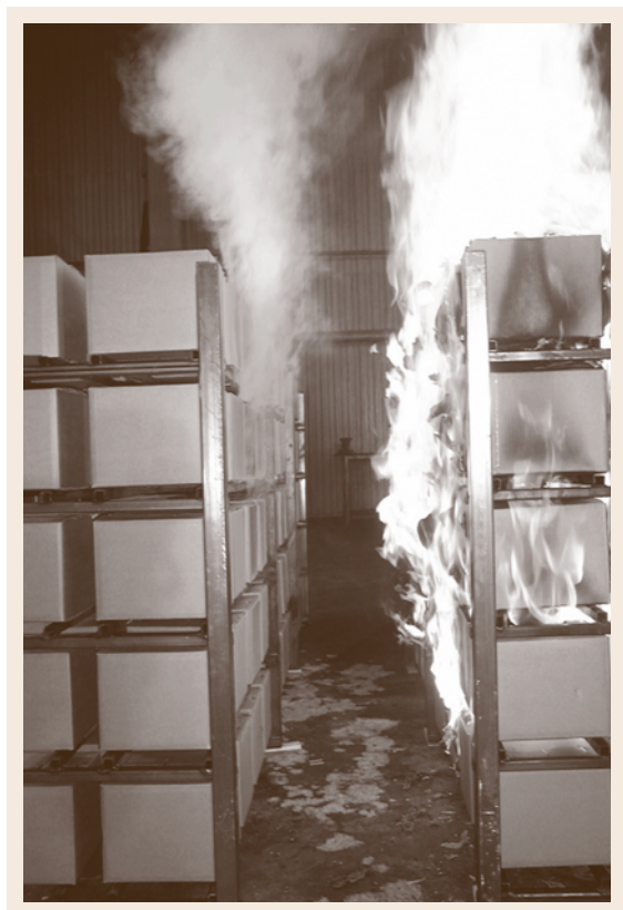
Fig. 15.29 Ignition of the left side cardboard boxes occurs when the combustible volatiles are leaving the surface at a sufficient rate (courtesy of SP)
