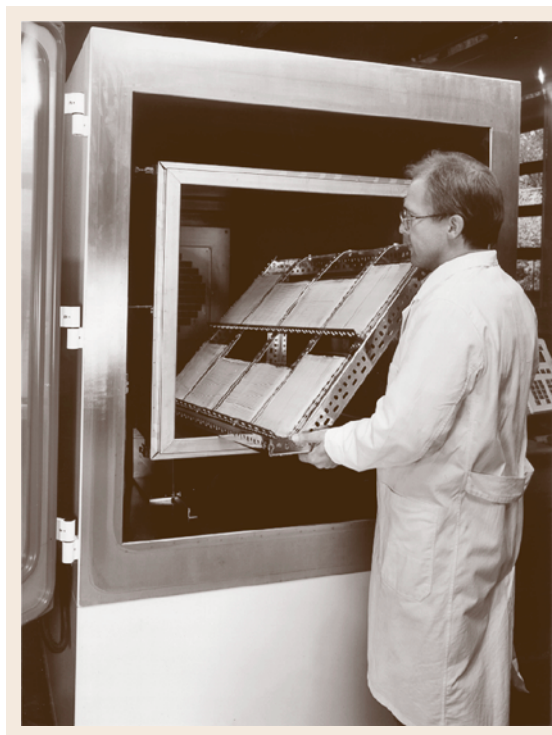
Fig. 15.18 1 m 3 emission test chamber loaded for a test with a flooring adhesive on glass plates (courtesy of BAM)
