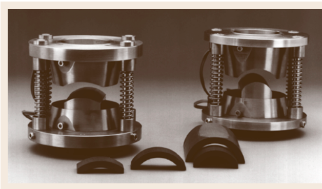
Fig. 10.5 Segment poles with pole coils
