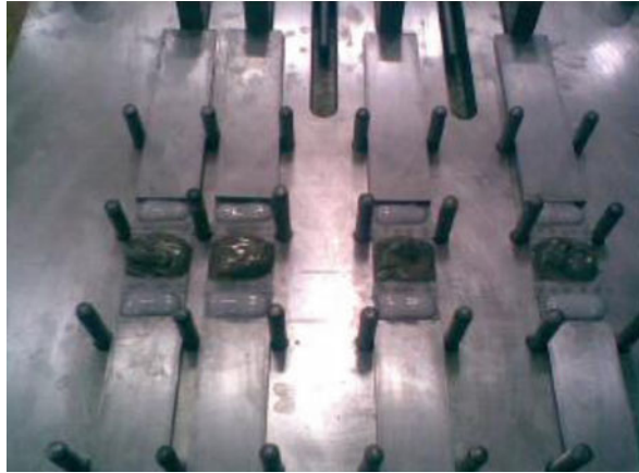
Fig. 4 Manufacture of mixed adhesive joints [7]
