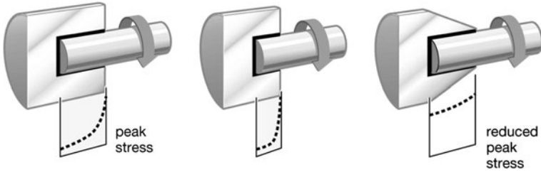
Fig. 8 Stress distribution across bond
