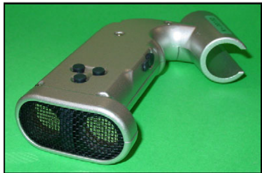
Fig. 4. K-Sonar ultrasonic sensor is designed with a mount point to fit on a blind person’s long cane
