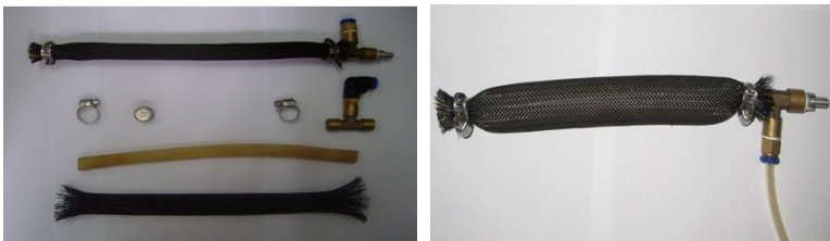
Fig. 1. Materials of pneumatic muscle actuator and pneumatic muscle actuator made in lab
