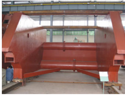
Fig. 3. Wall frame of the manipulator
