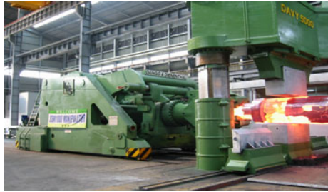
Fig. 1. The working environment of forging manipulator
