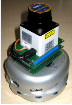
Fig. 8. Khepera III with mounted Hokuyo's LRF
