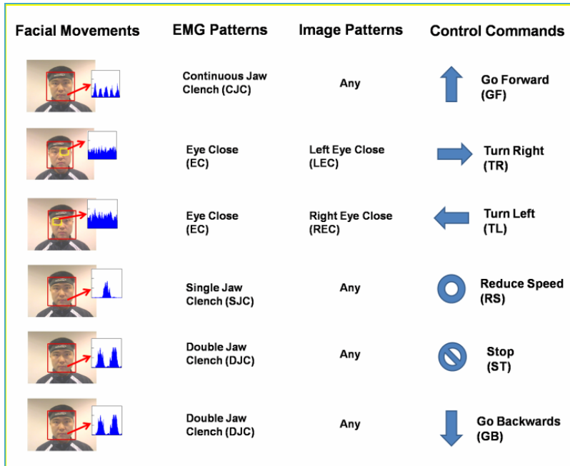
Fig. 4. Diagram showing sample face control movements and control strategy of EMG and visual based control methods
