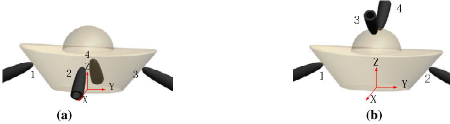
Fig. 5. Gold ingot gripped by four (a) PCwF (b) SFC
