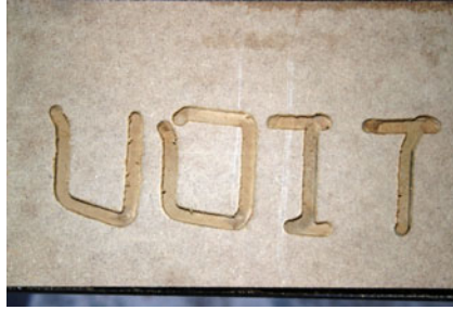
Fig. 7. The characters cut by the portable multi-Axis CNC
