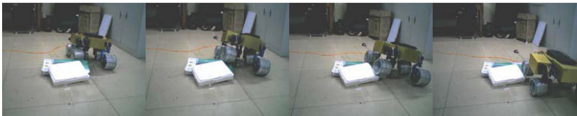
Fig. 15. Five diamond wheel type configuration through the rough ground test ( \alpha_l = -18^\circ and \alpha_b = 18^\circ )
