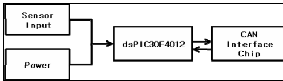
Fig. 8. Hardware structure of CAN communication module
