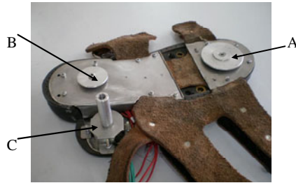
Fig. 3. The sensing shoe of ELEBOT. A, B and C are the force sensor in the shoe.
