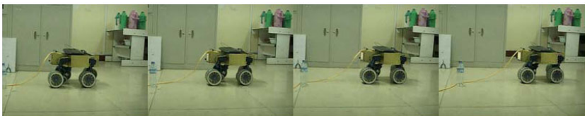
Fig. 14. Diamond-shaped configuration of five straight wheel class performance test ( \alpha_l = -18^\circ and \alpha_b = 18^\circ )
