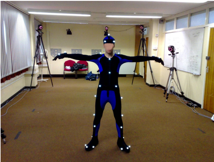
Fig. 4. Optical markers placement - front view
