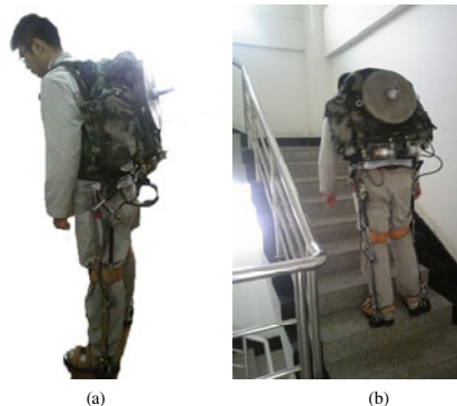
Fig. 7. The photos of ELEBOT in experiments. (a) ELEBOT supported 30 kg payload when the operator was standing. (b) ELEBOT went up stairs with 30 kg payload following the operator.
