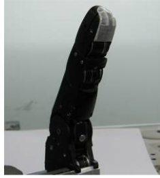
Fig. 1. Finger of the HIT/DLR Hand II dextrous robot hand with the finger-tip flexible tactile sensor
