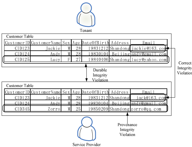
Fig. 1. A Simple example of data integrity in SaaS model
