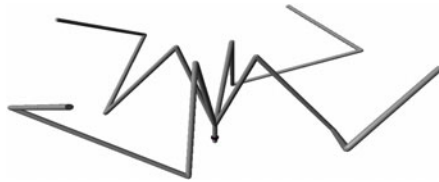
Fig. 4. Three-dimensional figure of the four-branch antenna
