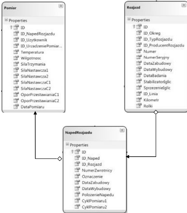
Fig. 4. Detailed structure of the “Measurement”, “Switch” and “Switch point mechanism” tables with their interrelations
