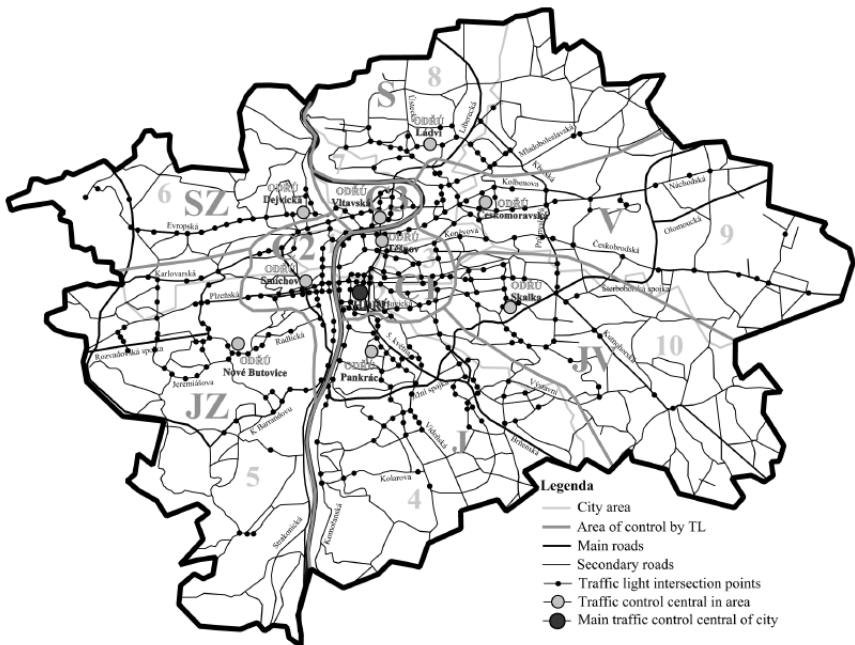
Fig. 1. Schematic layout of TCC in area in Prague with new area marking
