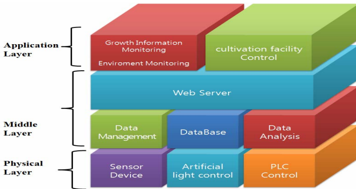
Fig. 3. Paprika Green House System Structure
