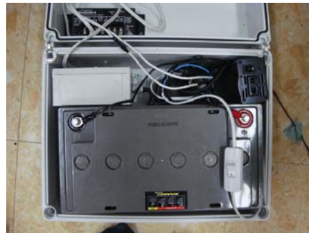
Fig. 8. salinity sensor receiver, integrated battery
