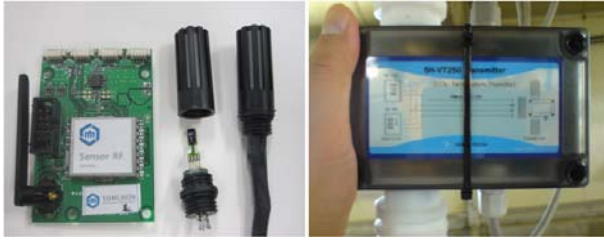
Fig. 2. Integrated sensor node and CO 2 sensor
