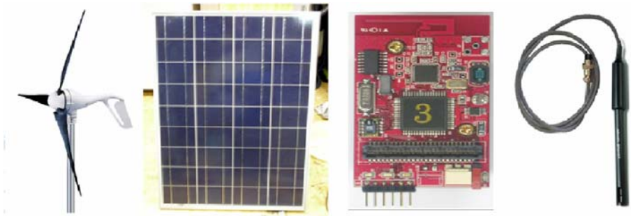
Fig. 6. Wind turbines, Solar cell, Network sensor node, temperature sensor in the SFMS
