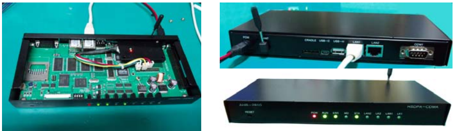
Fig. 3. Implemented MAP. The left figure shows internal circuit board, the right two figures shows the backside and the front of MAP respectively.
