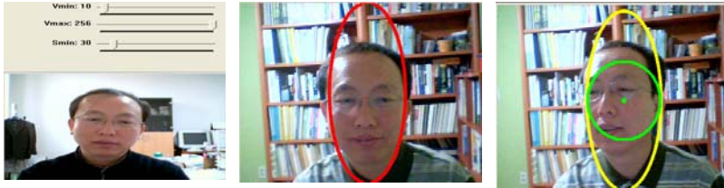
(a) manual setup of ROI (b) expansion of the tracked area (c) the proposed algorithm
