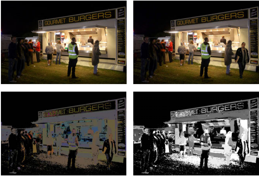
Fig. 8. Original image (top left) and tampered image (top right). At first glance, illumination map and distance map show plausible results on the tampered image. However, the illuminant estimates are obtained from the front of the woman, which is turned away from the restaurant lights. Therefore, the expected illumination should be more bluish, like e.g. at the back of the person in the middle.
