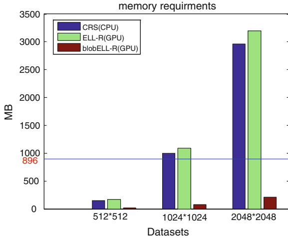
Fig. 41.4 Memory requirements of the different implementations for the datasets. The limit of 896 MB is imposed by the memory available in the GPU used in the work. The implementations needing higher amounts of memory than the value cannot run on this GPU. However, the use of the blobELL-R data structure reduces the demands, making most of the problems affordable
