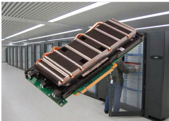
Fig. 1.1 The Tianhe-1A couples massively parallel GPUs with multi-core CPUs, employing 7,168 NVIDIA Tesla M2050 GPUs and 14,336 CPUs. It is a 2.507 Petaflop system consuming only 4.04MW
