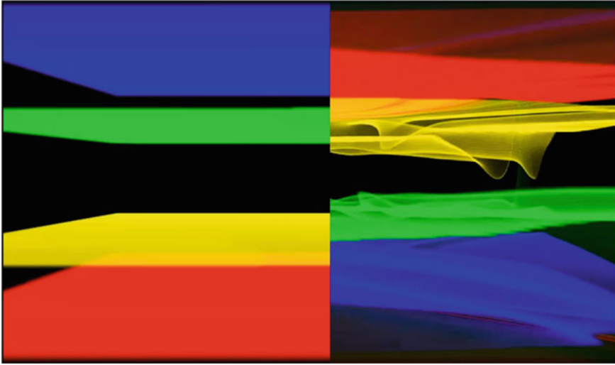
Fig. 22.5 Boss transition of the temperature field in 3-D, using isosurfaces at Ra = 10^7 . When temperature is normalized to the interval between zero and one, red displays a temperature of 0.9, yellow a temperature of 0.75, green a temperature of 0.25, and blue a temperature of 0.1. The left half of the figure is the visualization at initial condition, while the right half is a time shortly thereafter
