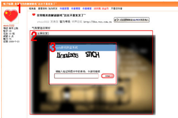
Fig. 7. Instance of flash-based CAPTCHA phishing: 1 is a post in web forum; 2 is the phishing flash which exhibit a game; 3 is the CAPTCHA input panel which shows: please enter the two words to make game continuing
