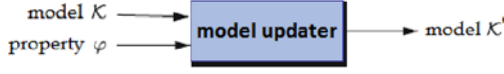
Fig. 4. Model updater receives \mathcal{K} and \varphi and returns an updated model \mathcal{K}'
