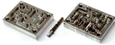
Fig. 1. Effects of cutter deterioration until breakage in machining. Image © Prof. Shea TUM PE.
