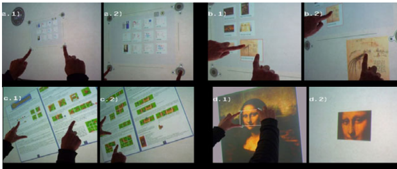
Fig. 2. a) Whole widget Manipulation b) Drag and Drop c) Flip Pages d) Crop
