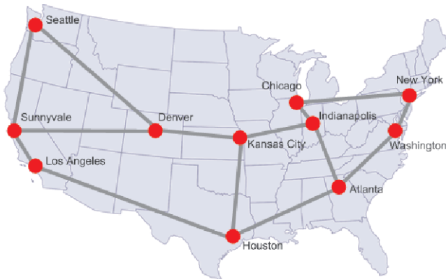
Fig. 2. Backbone hubs on the Internet2 network and traffic flow links between them
