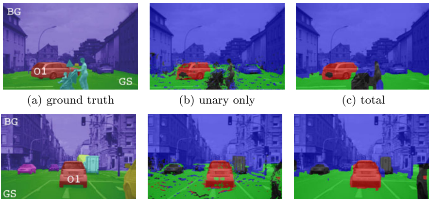
Fig. 5. Segmentation results of STROLLER (top) and LEAD_VEHICLE (bottom) scene. Middle: Result if data is evaluated for each pixel independently. Right: Result if smoothness and global ordering constraints are incorporated via local neighborhood inference (result after 40 iterations of loopy belief propagation).
