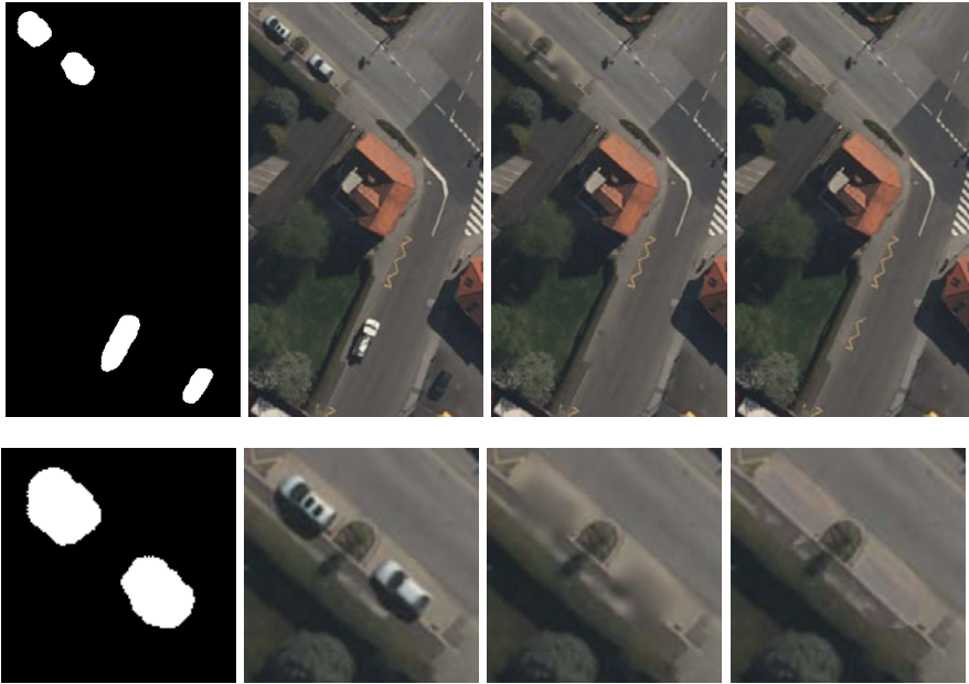
Fig. 4. Inpainting results using a car detection mask. From left to right: The car detection mask, the fusion result computed without using a car detection mask, the result obtained by pure inpainting and the inpainting with supporting exemplars. The car areas are successfully removed in both cases, however the exemplar-based fill-in appears more naturally. Best viewed in color.
