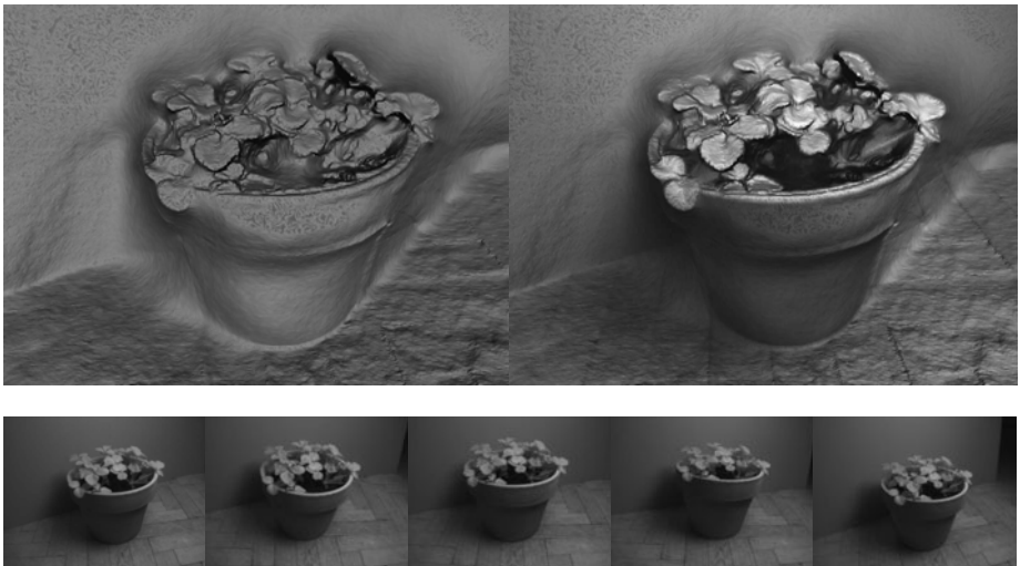
Fig. 1. Dense depth maps computed from images of a hand-held camera
