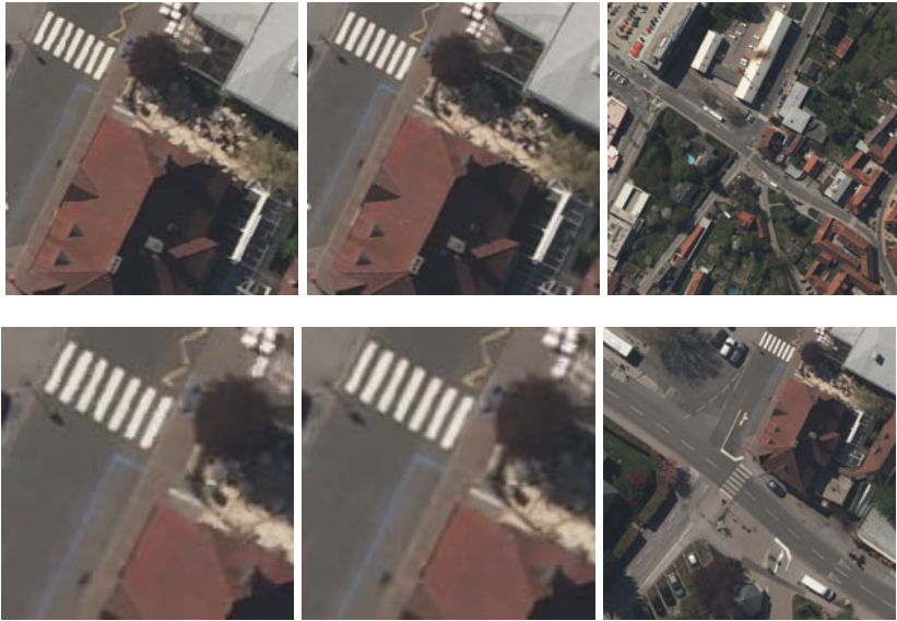
Fig. 3. Some fusion results. The first column shows results obtained with the TV-L^1 model (three input observations). The second column depicts corresponding images computed with our fusion model using a DTCWT regularization, which yields images with an improved natural appearance ( \lambda = 1.0 ). Larger fusion results are given in the third column, where we exploit a redundancy of ten input images. The color fusion ( 1600 \times 1600 pixels) can be obtained within two minutes. Best viewed in color.
