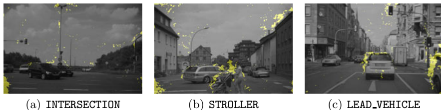
Fig. 3. The test scenes (mask: pixels w/o scene flow data, e.g. due to stereo occlusions).
