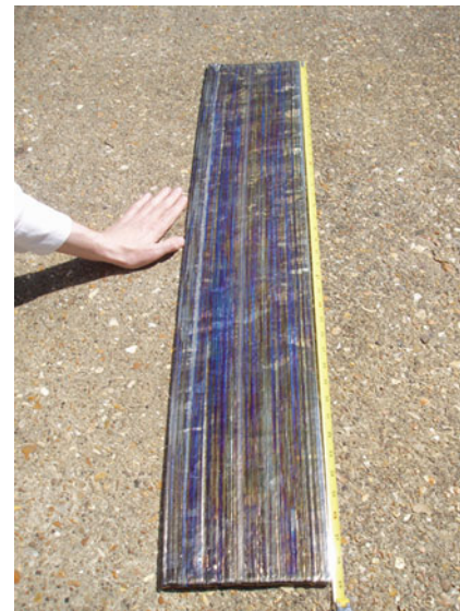
Fig. 3 1000 mm × 200 mm × 4 mm RUAM titanium wall structure
