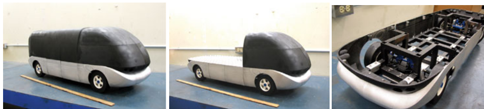
(b) A 1:5 scale model built using FDM (fused deposition modeling) rapid prototyping
