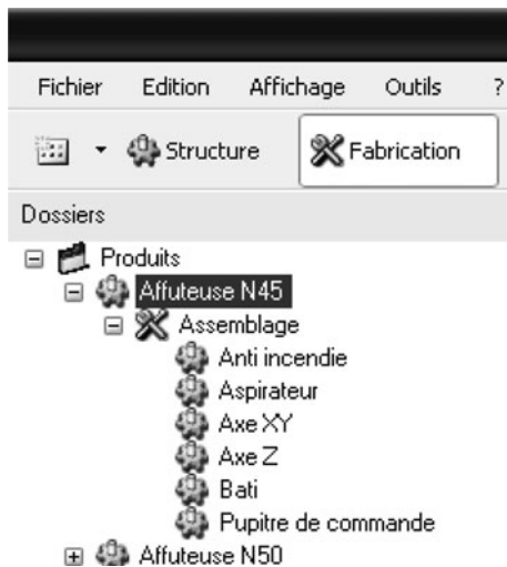
Fig. 10 Manufacturing decomposition of a grinding machine
