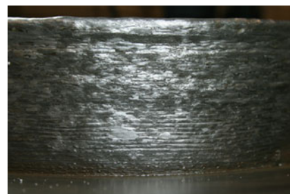
Fig. 1 Layer structure of a wire based additive layer manufacturing part
