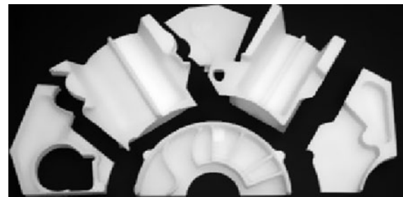
Fig. 6 Drag casting pattern FDM modules
