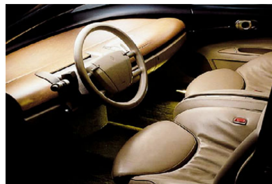
Fig. 6 Recyclable dashboard of a Renault concept car
