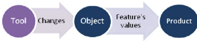
Fig. 1 An example of ENV application for a motion description: “a tool moving an object”, is a tool that changes the value of the object’s (E) speed (N) from zero (V1) to a certain value (V2) measured in km/h
