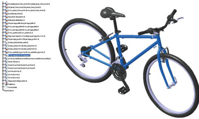
Fig. 9 CAD model of a configured bicycle
