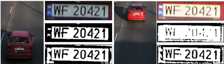
Fig. 2. Example of licence plate thresholding. The images show a car captured in shadow and sunshine. By side presented are the extracted plates (top) and effects of constant thresholding (middle - notice the right plate is unreadable) and adaptive thresholding (bottom - both plates are readable).
