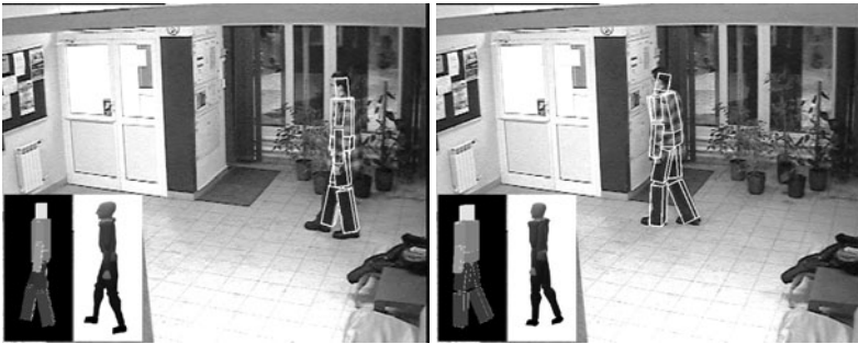
Fig. 2. 3d model-based human body tracking, frames #5, #40, left bottom: appearance images of person undergoing tracking. The overlap degree between the appearance image and the projected model into 2d image plane is 0.84 and 0.86, respectively.
