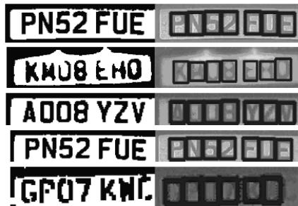
Fig. 5. Number plate cropped and characters detected during day time, night time, sunny and cloudy condition, respectively
