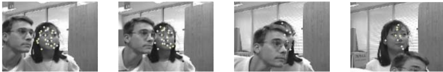
Fig. 3. Tracking a face that undergoes occlusion by an another face. Frames #420, 422, 434, 449.
