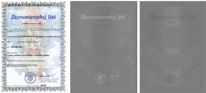
Fig. 5. Sample document containing a stamp (left), C_b and C_r component of its YC_bC_r representation (right)
