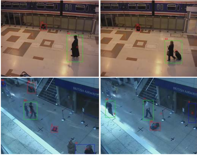
Fig. 3. Example detection presented on PETS 2006 (upper row) and PETS 2007 (lower row) data. Left luggage is marked with red rectangle, while moving humans are marked green; false objects are marked with blue rectangles.
