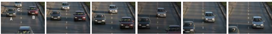
Fig. 5. A typical sequence of images acquired by our system. Car A is being overtaken by cars B and C. It is clear that car A is the slowest and car B is the fastest among the three. Moreover, car A is maintaining a constant velocity of 45 \pm 1 km/h as measured by an onboard GPS device. Velocities of cars B and C are unknown. The average measured speed in km/h returned by our system is: 46,0 (A), 83,7 (B), 62,9 (C).
