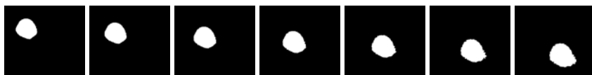
Fig. 4. Interpolation of markers – the first and the last are binary images showing results of the coarse segmentation and computed using EF images, while all the others are results of morphological interpolation using initial position from first and final position from the last image
