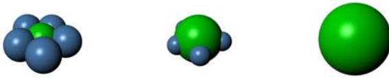
Fig. 3. Progressive merging (from left to right): a fraction of mass is transferred to a particle from its neighbours at successive time steps
