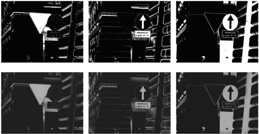
Fig. 3. Results of image segmentation with the fuzzy k-means for \gamma = 1.4 : The probability fields (upper row). These filtered with our version of the anisotropic diffusion.
