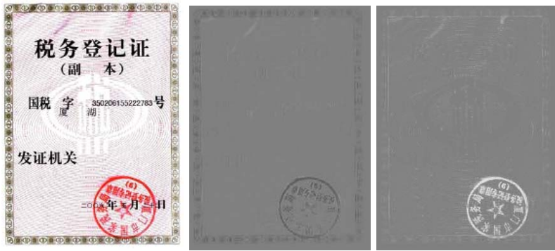
Fig. 4. Sample document containing a stamp (left), C_b and C_r components of its YC_bC_r representation
