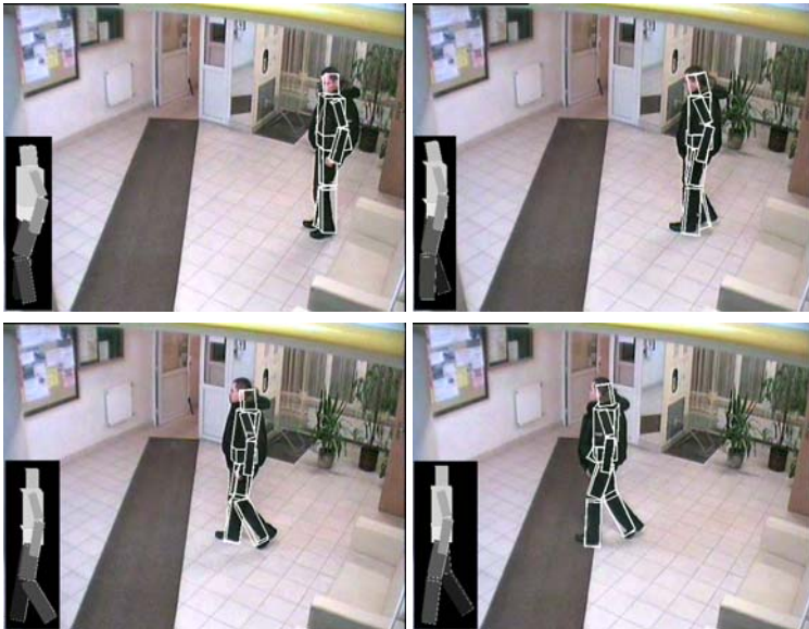
Fig. 1. 3d model-based human body tracking, frames #5, #15, #25 and #35, left bottom: appearance image of person undergoing tracking. The degree of overlap between the appearance image and the projected model into 2d image plane of the camera is 0.86, 0.80, 0.80 and 0.79, respectively.
