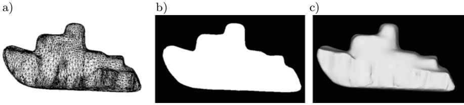
Fig. 5. Triangle mesh model of the battleship: a) mesh, b) two-colour rendering, c) the 3D look after rendering by the lighting
