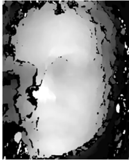
Fig. 4. Disparity map of a left face from Fig. 3. Higher intensity corresponds to bigger disparity.
