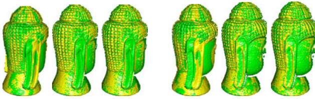
Fig. 4. Registration results for our HM-ICP algorithm applied to different overlapping range images using different values of m . Left three: buddha140-120; Right three: buddha120-100. In each case: m = 1 , m = 16 , m = 25 .
