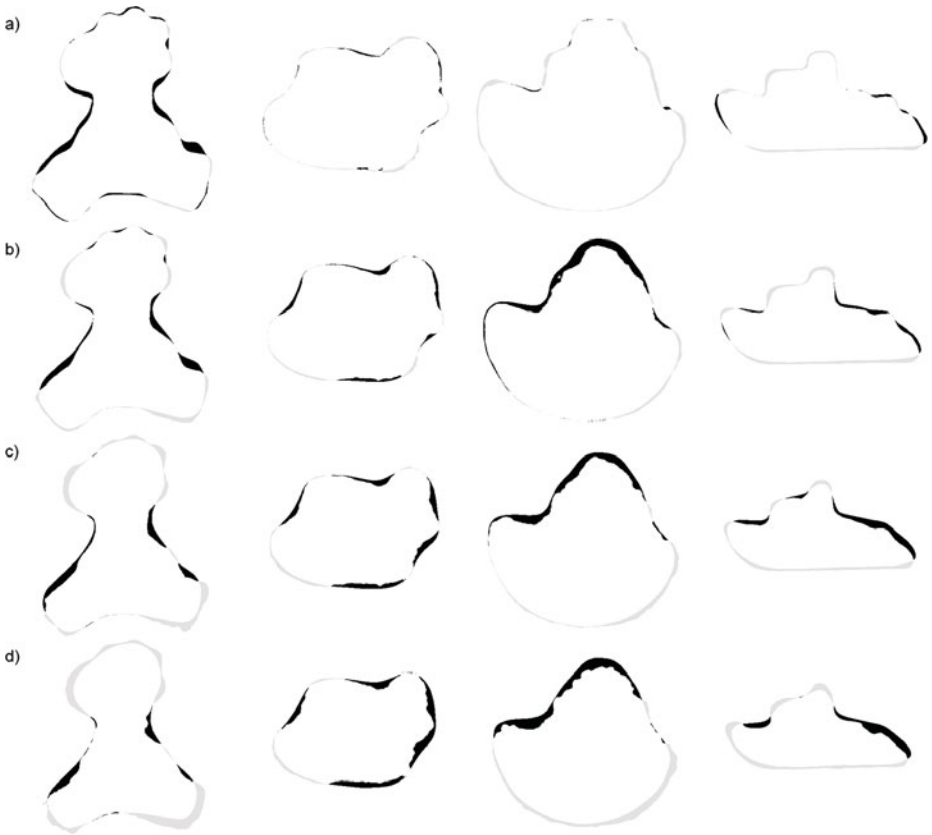
Fig. 7. The contour's similarity: a) P_1 , b) P_{33} , c) P_{67} , d) P_{100} ; grey - the real object's contour ( S_A ), black - the virtual object's contour ( S_B ), white - the common part of contours ( S_I )
