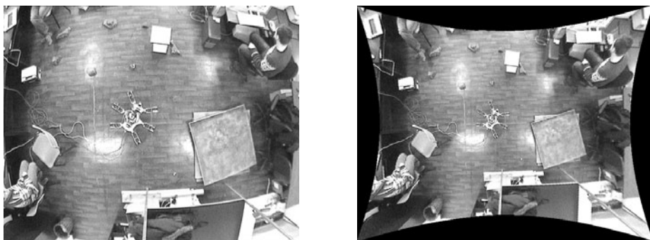
Fig. 3. The exemplary view from the ceiling camera before (left) and after (right) undistortion
