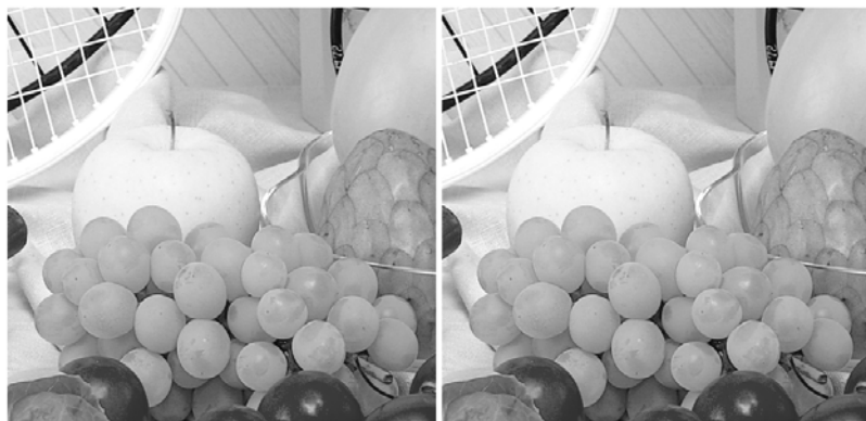
Fig. 6. The image Fruits; a) input, b) result - 11% of edge points, 15% of random points, MSE=20.65
