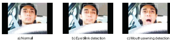
Fig. 3. Example result of the eye blink and mouth yawning detection
