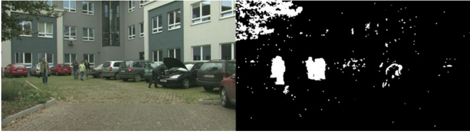
Fig. 4. Motion map (right) obtained for exemplary frame (left) (white pixels moving, black pixels steady)
