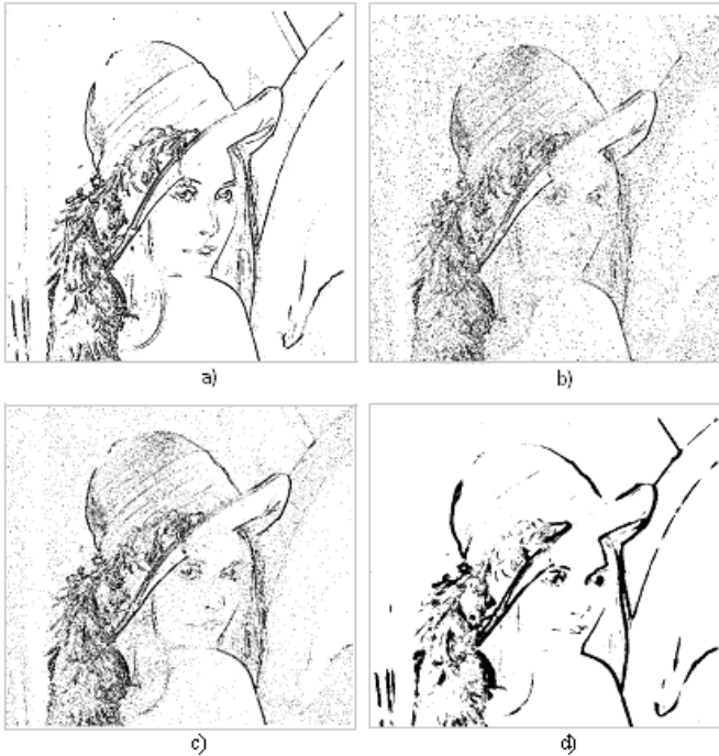
Fig. 1. The 9-10% pixels with the highest evaluation according to the presented operators, a) Roberts, b) Laplace4, c) Laplace8, d) Gauss
