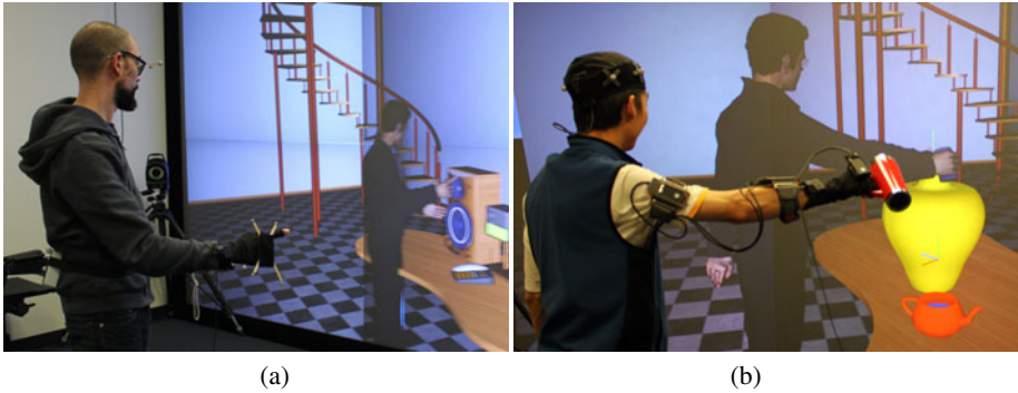
Fig. 2. The figure shows (a) the camera-based motion interface and (b) our gesture vest interface based on inertial sensors [10]
