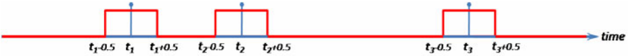
Fig. 2. t_1, t_2, t_3 are the time spots when a participant gives backchannel feedback in a parasocial interaction. A 1.0s window of opportunity is put around each timestamp so that the time spot is in the middle of the window. The samples within the window are set to 1 to indicate the presence of feedback, while others are set to 0.
