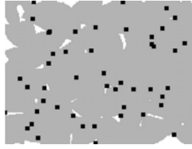
Fig. 7. Area covered by 48 sensors having a limited 90^\circ sensing range, using CMA-ES optimization. The terrain is the small map presented in Fig. 4. Dark spots are sensor positions, grey areas are covered by sensors, while blank areas are the uncovered area.
