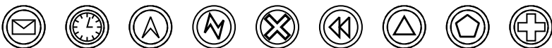
Fig. 9.14 Intermediate Catch Events – Message, Timer, Escalation, Error, Cancel, Compensation, Signal, Multiple, Parallel Multiple
