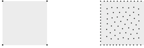
Fig. 1. Best distributions found by the hill-climber, for the sum of pairwise distances diversity measure (left) and the Solow-Polasky measure (right)
