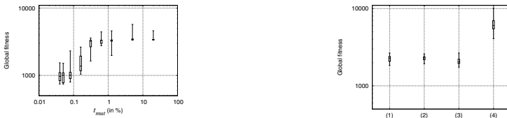
(a) When the initial population size is 625 flies, and depending on t_{mut} value. (b) When the initial population size is 160000 flies with: (1) constant \sigma = 0.1\text{mm} , (2) constant \sigma = 0.01\text{mm} , (3) t_{mut} = 0.0\% , and (4) t_{mut} = 0.05\% .
