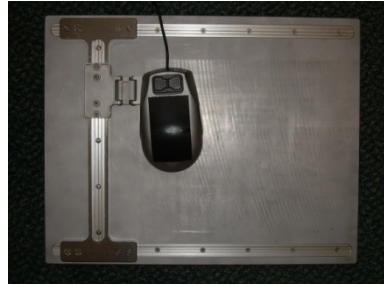
Fig. 4. Support aid for mouse enabling user to move vertically and horizontally in straight line
