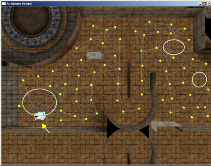
Fig. 3. Cognitive Topological map of Place Cells constructed by the robot while wandering into its environment using e_{max}^{Mp} = 40 and e_{max}^{Mte} = 20 .
