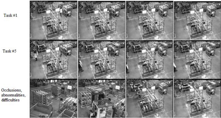
Fig. 1. Sequences from the dataset. The relatively low resolution and the several occlusions and self occlusions make very difficult the task of tracking thus necessitating holistic features and a robust model to recognize workflows. The first two rows depict two different tasks that would be difficult to distinguish even for the human eye; the third row shows some example frames of occlusions, outliers, and other challenges faced in this industrial dataset.
