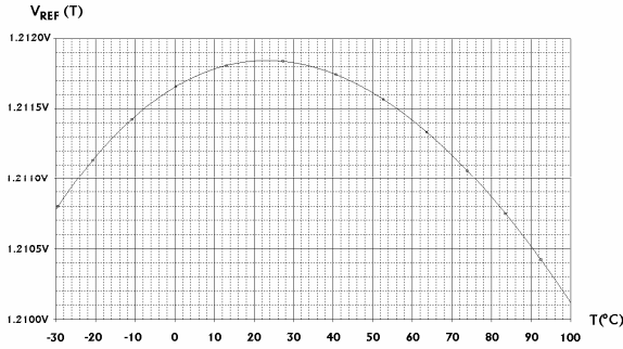
Fig. 11. The SPICE simulation for the superior-order curvature-corrected voltage reference
