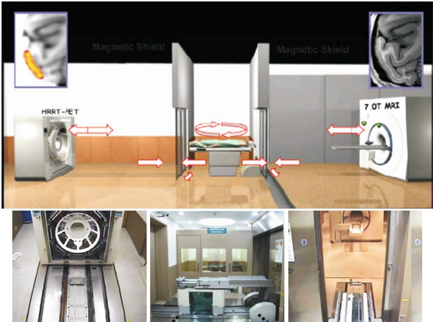
Fig. 2.10. PET/MRI fusion system. The system combines by two separate high-end imaging devices ( top ), the HRRT-PET ( left ) and the 7.0 T MRI ( right ) by means of a high-precision shuttle railway system ( bottom )
