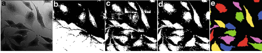
Fig. 1.26. Dynamic thresholding in microscopy [8]. The microscopy of a cell culture (a) was segmented using a global threshold (b), locally adaptive (c) and pixel-connected adaptive (d). According to morphological post-processing for noise reduction and a connected components analysis, the final segmentation is shown in (e)
