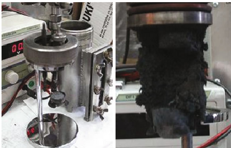
Fig. 29 Calorimetric bomb before ( left ) and after ( right ) the combustion synthesis in Si/PTFE system
