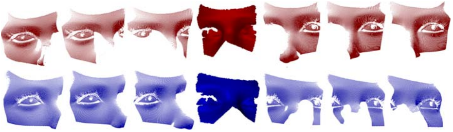
Fig. 2. 3D point clouds of the mannequin head at the seven positions. Left to right from -15 degrees to 15 degrees. Blue images represent the left camera and red images represent the right camera. The center images at 0 degrees are the reference surfaces.
