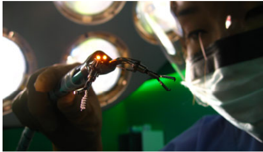
Fig. 1. Appearance of the tip of the scorpion shaped endoscopic surgical robot
