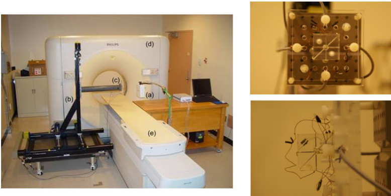
Fig. 2. Experimental setup (left) in CT scanner environment showing (a) Aurora field generator, (b) positioning system, (c) phantom mounted on a non-metallic extension arm, (d) CT gantry and (e) CT table. - Calibration phantom (right) with two 5-DOF sensors in each axis residing 10mm from each other.
