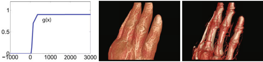
Fig. 2. A typical non-stationary opacity transfer function used for medical visualization (left). The transfer function is shifted along the x-axis to browse through different anatomical structures of a human hand (middle, right).
