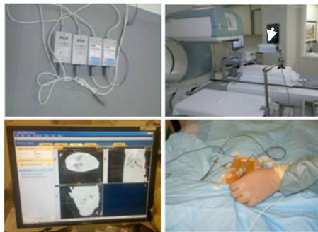
Fig. 1. Pictures showing various components of the real time 3D CT Image Guided Navigation System developed by our group: the upper left picture displays the connection trackers for EM tracking, the upper right picture shows the field generator that tracks the needle (white arrow). The bottom left picture shows the 3D image display available for the physician to design a pre-operative path planning in order to guide the needle to the tumor, and the bottom right picture shows the needle insertion inside the animal chest.
