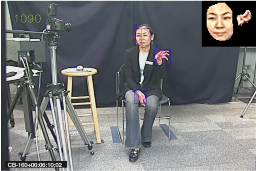
Fig. 1. Sample frame showing the tracked head (blob 0) and hands (blobs 1 and 2) of an interviewee. The tracker records the (x,y) coordinates, area and axis lengths of each detected blob. The skin color samples are shown in the upper right corner.
