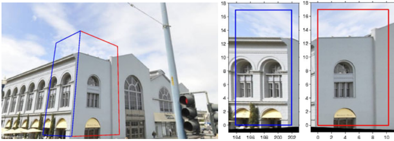
Fig. 3. Left: Building geometry projected into an image. Right: Two orthophotos generated from this image with overlaid geometry. The axes show the known scale in meters.
