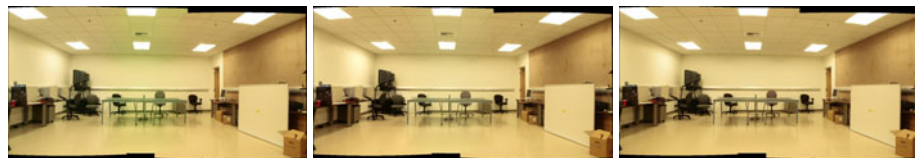
Fig. 11. Panorama generated from images captured by three different cameras, when using no color matching (left), inverse transformation for ideal devices (middle) and color matching using our method (right). The image on the left shows severe color mismatch. This is not corrected by the middle one – note the greenish tinge in the white of the floor and ceiling near the center and also lower saturation of the green color of the ping-pong table. These artifacts are completely removed by our method on the right. Please zoom in to see the differences.
