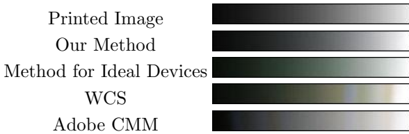
Fig. 9. Comparison of printer-to-projector color matching for a black-to-white gradient. Note that our method provides the closest match and the smoothest color transitions.
