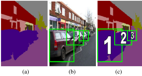
Fig. 2. (a) Object class segmentation results (without detection), (b) The detection result, (c) Combined segmentation and detection. Object class segmentation algorithms, such as [3], label all the cars adjacent to each other as belonging to one large blob. Detection methods localize objects and provide information about the number of objects, but do not give a segmentation. Our method jointly infers the number of object instances and the object class segmentation. See §2.3 for details. (Best viewed in colour)
