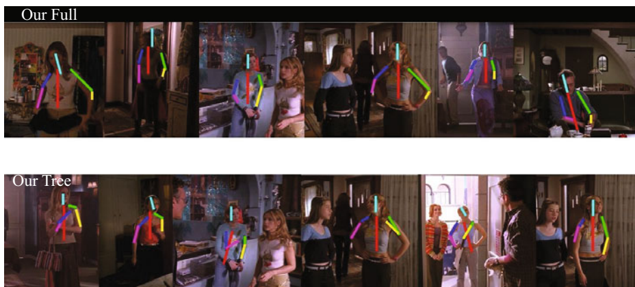
Fig. 4. Examples of stick-figure, upper body parses of figures in the Buffy produced by the full model trained on ours top row, and our tree model trained on ours bottom . Red: upper body; Green: head; Blue-Purple: left upper/lower arm; Green-Yellow: right upper-lower arm. Note doubled arms produced by the tree model, and the strong tendency for poses to have hanging arms.
