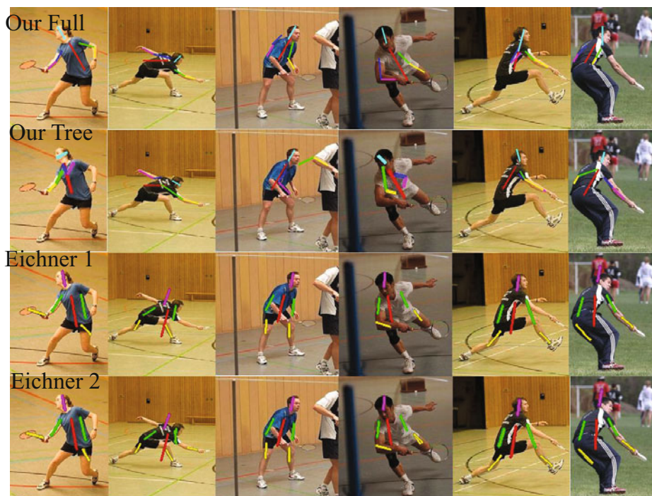
Fig. 5. Examples of stick-figure, upper body parses of figures in our dataset produced by the full model trained on our dataset top row, our tree model top-center and the code of Eichner et al. bottom center (trained on buffy_2to6) and bottom (trained on buffy_3&4 and pascal), all applied to our dataset. Red: upper body; Green: head; Blue-Purple: left upper/lower arm; Green-Yellow: right upper-lower arm. Note doubled arms produced by the tree model and a tendency for Eichner et al. to produce hanging arms, most likely a result of the strong geometric prior in their training datasets.
