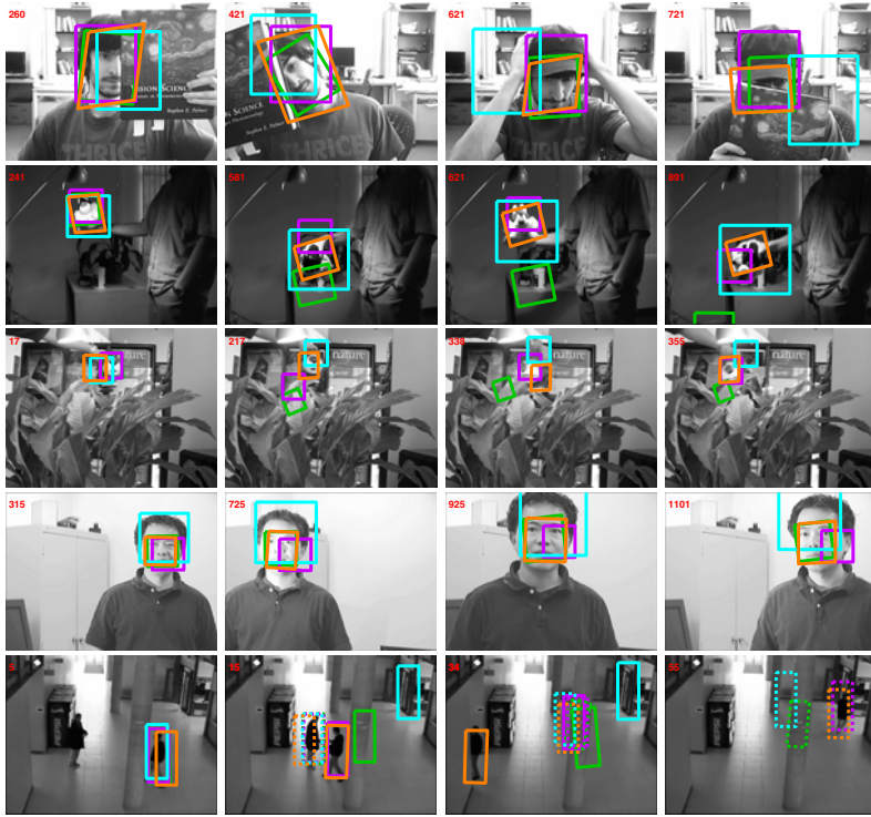
Fig. 4. Comparison to alternative trackers. Top-to-bottom as in Fig. 3. Orange, green, purple, and teal show results for proposed SOE, IVT, MIL, and MS trackers, resp.
