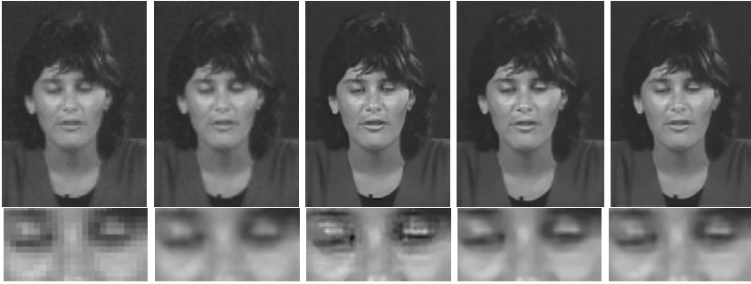
Fig. 8. Video super-resolution for Miss America sequence (frame 8, zoom factor 3, PSNR and SSIM in brackets). Left to right: NN(32.4259, 0.8580), BI(34.5272, 0.8958), GNL-Means(34.7635,0.9132), 3D-KR(35.53, NA), NL-KR( 36.6509, 0.9171 ). The GNL-Means method suffers from block effects, while our method is free from artifacts and is comparable to 3D-KR in this case.
