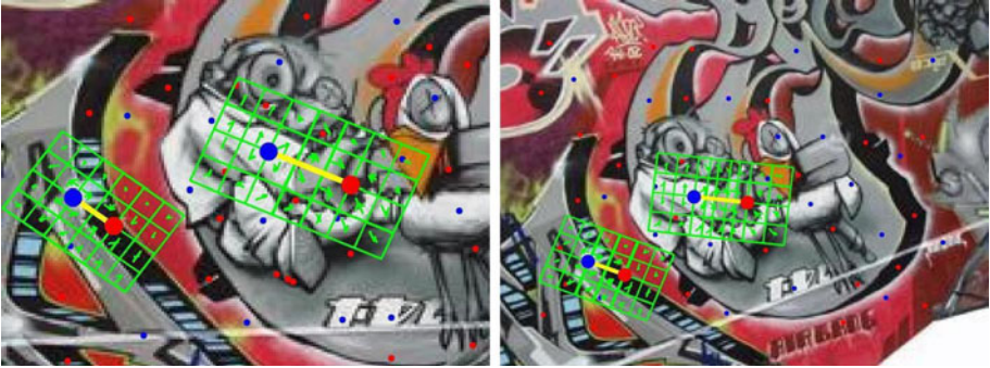
Fig. 6. The orientation and scaling for each feature point pair connected by an ascending path are uniquely determined through the direction and length of the line segments connecting minima and maxima. Images from [21]
