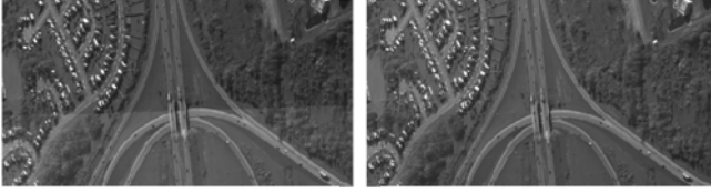
Fig. 9. This figure shows the result of multi-camera intensity equalization. Notice the seam in image on left which is not visible in equalized image on right.
