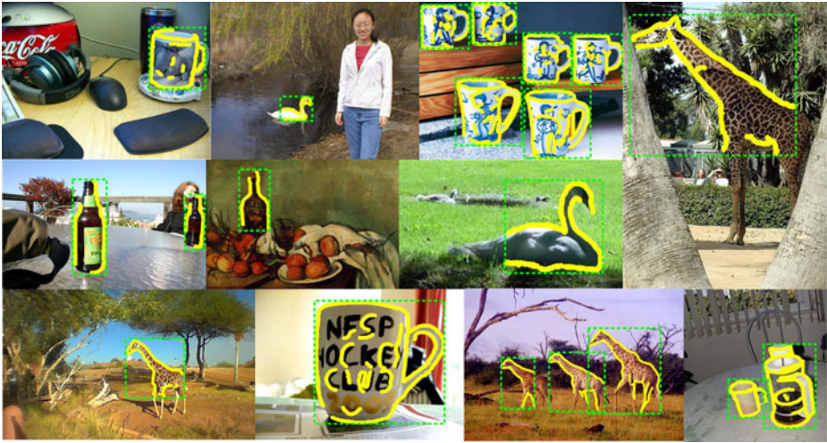
Fig. 6. Some selected results on ETHZ dataset [8] with the detected bounding boxes and contours plotted in green and yellow respectively
