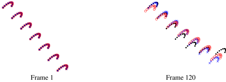
Fig. 2. Black dots \bullet represent the 2D measurements, red circles \circ a half-cylinder 3D shape registered by Algorithm 1 and blue crosses \times the results by the proposed Algorithm 2. The image data show the cylinder starting from a rest position in Frame 1 where the registration is perfect. The cylinder is bending at the last 3 semi-circles and the registration at the maximum deformation is strongly biased toward the deformation direction.
