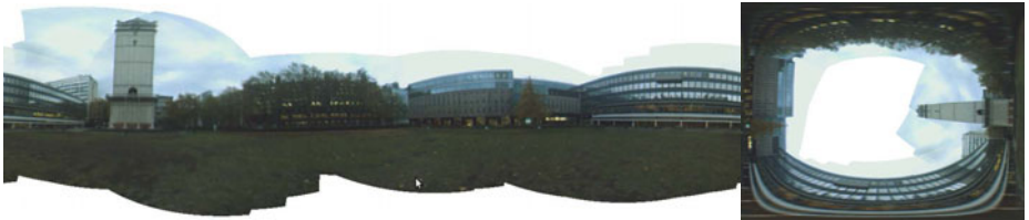
Fig. 5. 360^\circ Tower panorama from 21 keyframes (live hand held Unibrain webcam, 320 \times 240 resolution), shown in horizontally and vertically-oriented cylindrical projection. Note the vertical hole due to poor texture and cloud movement in the sky.
