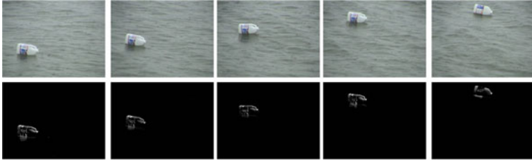
Fig. 4. Background subtraction by our method (no filter is performed on the results)
