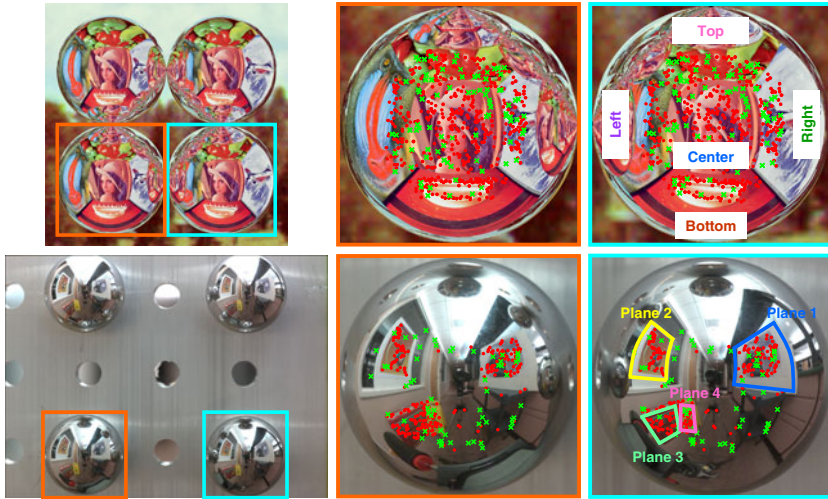
Fig. 4. Input images (left) and zoom-in of sphere images (middle and right) superimposed with extracted SIFT features. Red dots and green crosses respectively represent inliers and outliers determined in the iterative bundle adjustment process. Top shows rendered image using POV-Ray and bottom shows real photo captured using a camera.
