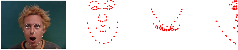
Fig. 7. a) A subject from the database. The white dots represent the manually annotated 2D points. b) Front, top and side views of the mean 3D shape reconstructed from the database.
