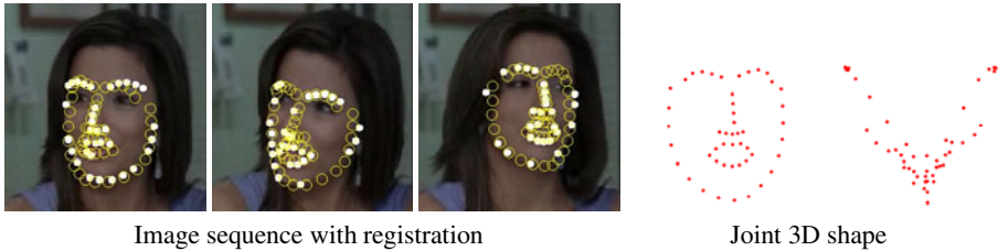
Fig. 10. The figures on the top show the image sequence together with the registration given by Algorithm 3 with 30% of missing data. White dots show the available 2D data while the yellow circles \circ represent the estimated registration. The three images on the bottom present front, top and side view of the joint 3D shape.
