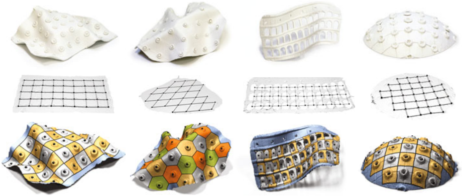
Fig. 4. Photographs of the plasticine imprints scanned in our experiments (top row), the detected grids in the parametrization domain obtained using MDS along with the locally refined grids (middle row), and the corresponding intrinsic structure depicted on the scanned models (last row). Parts of the shape that do not belong to any detected intrinsic regularities are in blue
