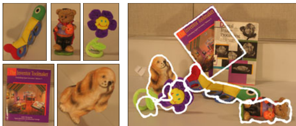
Fig. 7. Detecting objects. Templates, left, are matched to the image, right. Square patches are matched, searching over all rotations and scales, as described in Section 3.4. A similarity transform is fit to the resulting correspondences using RANSAC.
