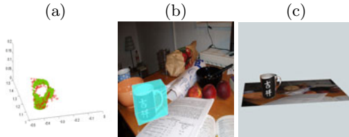
Fig. 2. Point clouds (green) from a 3D model is registered to the inferred partial 3D point cloud (red) by DEHV (a). This allows us to achieve an accurate 6 DOF pose estimation (b) and realistic 3D object modeling (c).
