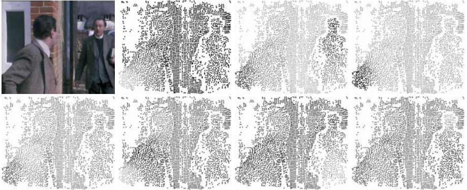
Fig. 4. From left to right, top to bottom: (a) Input frame. (b-h) The first 7 of m = 13 eigenvectors. Clearly, the eigenvectors are not piecewise constant but show smooth transitions within the object regions. However, discontinuities in the eigenvectors correspond to object boundaries very well. This information needs to be exploited in the final clustering procedure.
