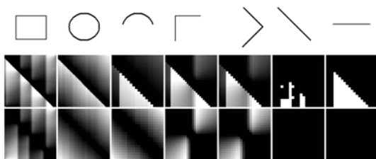
Fig. 3. Visualization of descriptors for selected contour primitives. Middle row shows descriptors from [25] and bottom row shows our descriptors. Note how each fragment is included in its respective closed contours (square and circle) in our version, which is not fulfilled for [25] since it was designed for closed contour matching.
