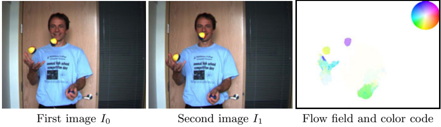
Fig. 7. When employed for optic flow, the proposed method can successfully capture large displacements without the need for coarse-to-fine approaches, since a global optimization is performed over all labels. In contrast to existing methods, our solution is within a known bound of the global optimum.
