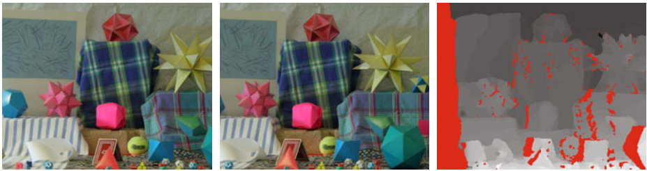
Fig. 6. The proposed method can be employed to simultaneously optimize for a displacement and an occlusion map. This problem is also too large to be solved by alternative relaxation methods on current GPUs. From left to right: (a) Left input image I_L . (b) Right input image I_R . (c) Computed disparity and occlusion map, red areas denote occluded pixels.
