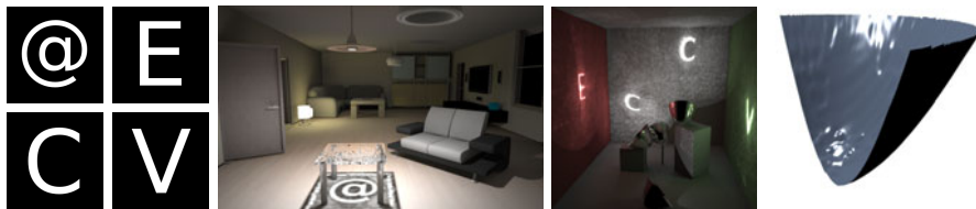
Fig. 1. The left image shows four of our optimization targets for which we generated geometry with our proposed optimization approach. The second and third image show a physically correct light transport simulation illustrating the results. For the living room scene we optimized a glass table to cast the predefined caustic. The letters E C C V in the right image are caustics from parabolic reflectors with a small embedded light source. The last image shows one half of such an optimized parabolic reflector.
