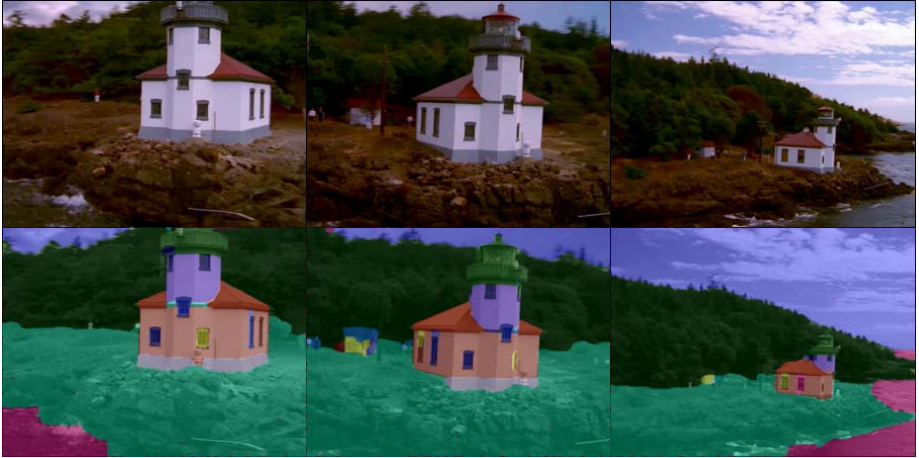
Fig. 1. Results from the on-line, unsupervised, photometric segmentation of a video sequence with MHVS. Top: original frames. Bottom: segmented frames. MHVS keeps track of multiple possible segmentations, collecting evidence across several frames before assigning a label to every pixel in the sequence. It also automatically creates and terminates labels depending on the scene complexity and as the video is processed.
