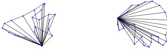
Fig. 1. Examples of fan-shaped triangulation. The boundaries of the shapes are highlighted in blue, and the frame edges are indicated in black.
