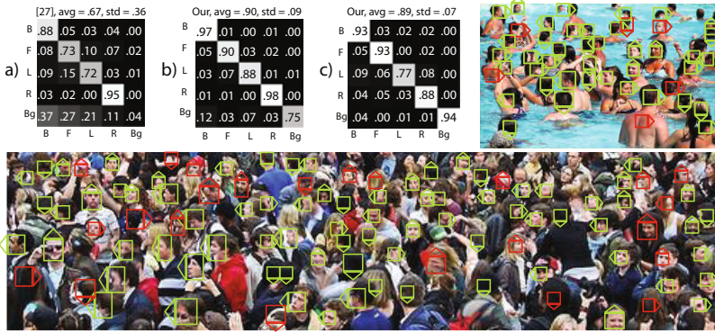
Fig. 4. Confusion matrices for the experiments on head pose detection and classification. In (a) e (b), results for the first experiment on 4 Pose Head dataset (Orozco’s method in (a) [29], our method in (b)). (c) is the result of the second experiment with the more general dataset (see text for details). The other images are examples of detection and classifications in crowded scenes. The arrows indicate the head orientation. In green the correct answers provided by classifier, in red the misclassifications.
