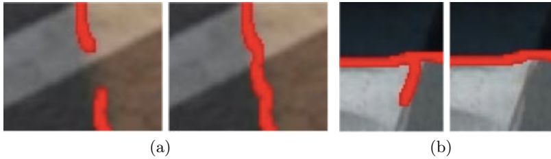
Fig. 2. Creating shadow contours by enforcing local consistency. Our CRF formulation may help to (a) bridge the gap across X-junctions where the local shadow classifier might be uncertain, and (b) remove spurious T-junctions which should not be caused by shadows.
