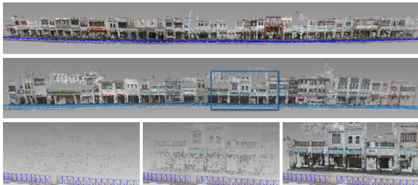
Fig. 4. Canton sequence. Top row is the complete reconstruction of Canton#1 with resampled 3D points. Middle row is the complete reconstruction of Canton#2 with resampled 3D points. Bottom row is a close up view of the blue rectangular region of the middle row in three different resample rates 5%, 20% and 100%.
