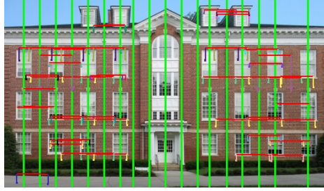
Fig. 2. An example of detected repeating features and symmetry axes. Only the feature pairs for the strongest repetition interval are displayed. It can be seen that the symmetry axes are repeating at half the interval of the window repetition.
