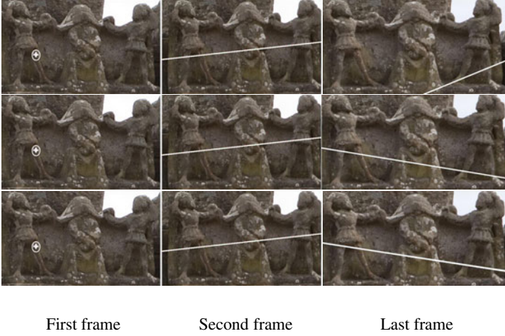
Fig. 2. This figure illustrates the improvement achieved at each step of our algorithm. If the cameras are reconstructed without imposing loop constraints, the epipolar lines between the first and the last frames are extremely inaccurate (1st row). They become much more accurate when the constrained optimization is performed (2nd row). Finally, the result is almost perfect once the homography registration is done.
