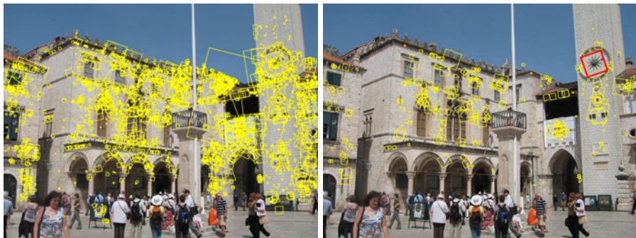
Fig. 1. SIFT Features in an image corresponding to reconstructed 3D points in the full model (left) and the compressed model (right) for Dubrovnik. The feature corresponding to the most visible point (i.e., seen by the most number of images) is marked in red in the right-hand image. This feature, the face of a clocktower, is intuitively a highly visible one, and was successfully matched in 370 images (over 5% of the total database).
