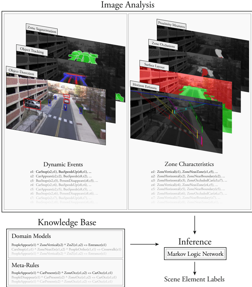
Fig. 1. System overview. Our scene understanding system consists of an image analysis module (Section 3) that takes an input video and outputs a set of events and zone characteristics as observational evidence, a knowledge base (Section 4) that stores human elicited domain models and general rules about scene geometry and occlusion as a set of first-order logic rules, and an inference engine (Section 5) based on Markov Logic Networks that uses the logic rules and observational evidence to infer the labels of visible scene elements.
