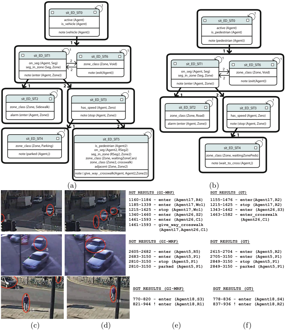
Fig. 6. SGT used to interpret behaviors of (a) vehicles and (b) pedestrians. (c,d) Selected frames from each interval. Semantic predicates are generated deterministically using (e) the learned region maps and (f) their corresponding GT maps.
