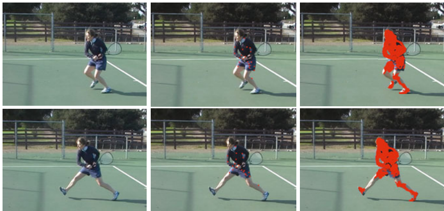
Fig. 4. (Top) Frame 490 of the tennis sequence with (left) actual image, (middle) KLT points and (right) LDOF points. (Bottom) Frame 495 of the sequence with (left) actual image, (middle) KLT points and (right) LDOF points. Only points on the player are marked. KLT tracker points are marked larger for easy visual detection. Figure best viewed in color.
