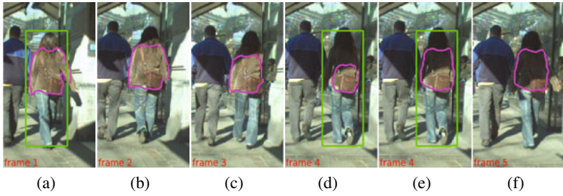
Fig. 4. Adaptation to lighting changes: (a-c) tracked shape becomes too small due to lighting changes; (d,e) level-set re-initialization is triggered; (f) tracking can continue.
