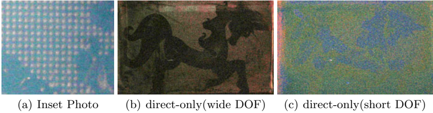
Fig. 10. Direct-only images by Nayar et al. [1] method for a horse-shaped object enclosed in an aquarium with diluted milk(Concentration 0.11%) (a) Inset of a captured photo with a projected high-frequency pattern (b) Direct-only image with wide projector’s DOF (c) Direct-only image with short projector’s DOF
