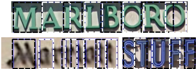
Fig. 7. This figure shows some advantages of using part based object detection. In the images of ‘MARLBORO’ and ‘STUFF’, character segmentation is extremely challenging because of the cast shadows and letter designs. Using the character detection approach allows us to avoid explicit segmentation and instead relies on local peaks from our character detector. The configuration of the word ‘Marriott’ shows how a pictorial structure model is tolerant of minor errors in the part detections. We can see that even though the first ‘r’ is not in the correct position, the total configuration cost for the word is better than that of the others associated with that image.
