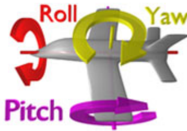
Fig. 2. Possible rotations around the 3 axes
