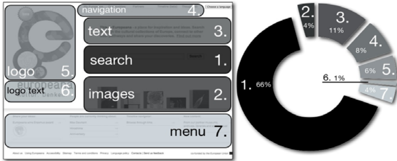
Fig. 1. a. Europeana 'home screen' augmented by AoI. b. Doughnut graph showing percentage of fixation for each AoI on 'home screen'.
