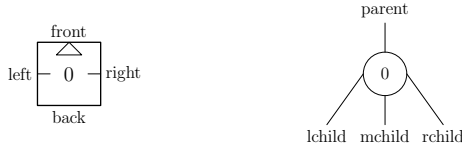
Fig. 3. A robot and its graphical node counterpart. The hinge joint is on the left-right axis.
